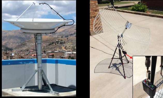
“Professional” (Left) & Low Cost (Right) HRIT/EMWIN Antennas
