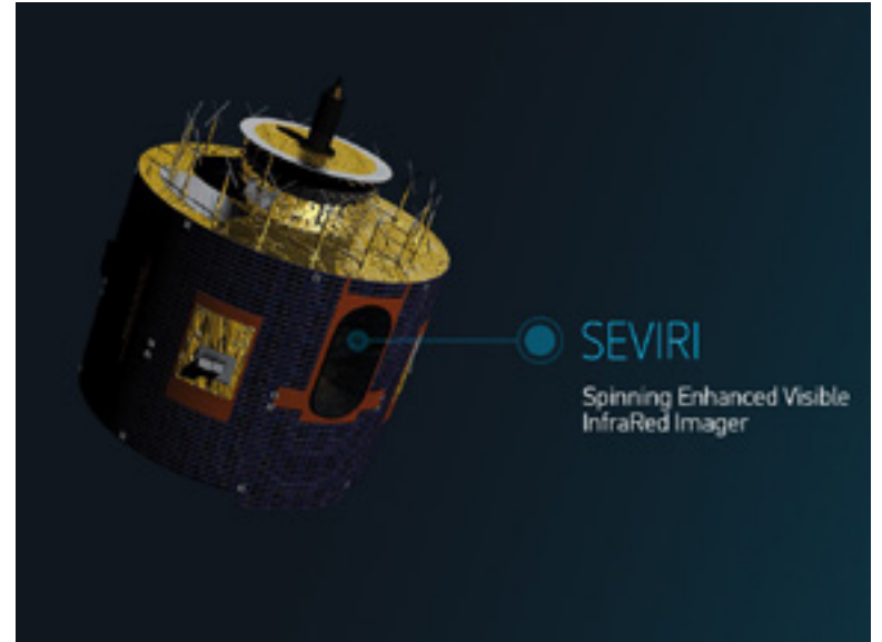
Clockwise from top left: ATMS and CrIS sounders onboard JPSS polar-orbiting satellites; IASI, MHS, and AMSU-A sounders onboard EUMETSAT's MetOp polar-orbiting satellites; SEVIRI onboard EUMETSAT's Meteosat geostationary satellites; and ABI onboard NOAA GOES geostationary satellites.
